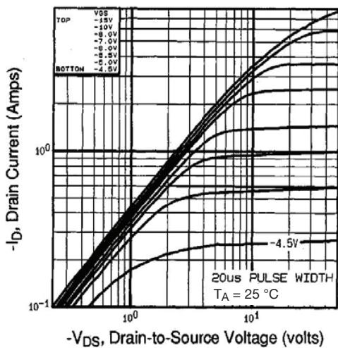
Fig. 1 - Typical Output Characteristics,  $T_A = 25$  °C
