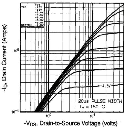
Fig. 2 - Typical Output Characteristics,  $T_A = 150$  °C
