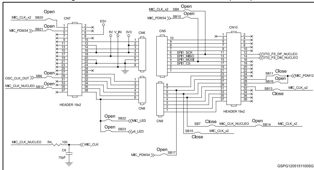
Figure 3: X-NUCLEO-CCA02M1 circuit schematic (Part 3)
