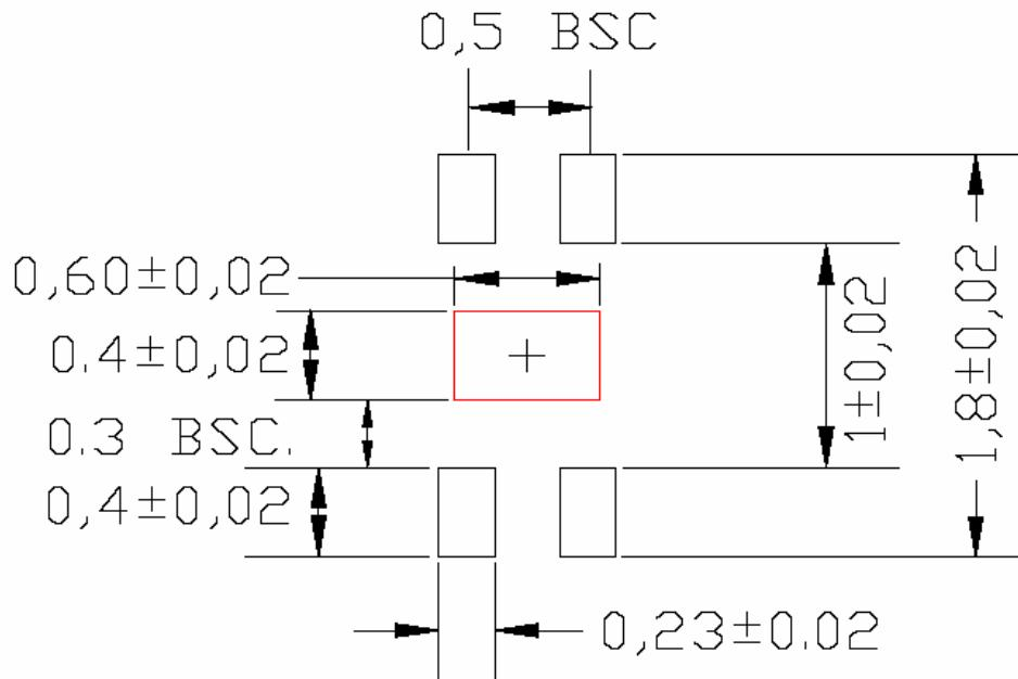
Optional for maximum thermal performance, heatsink should be connected to GND plane of PCB for maximum thermal performance.
