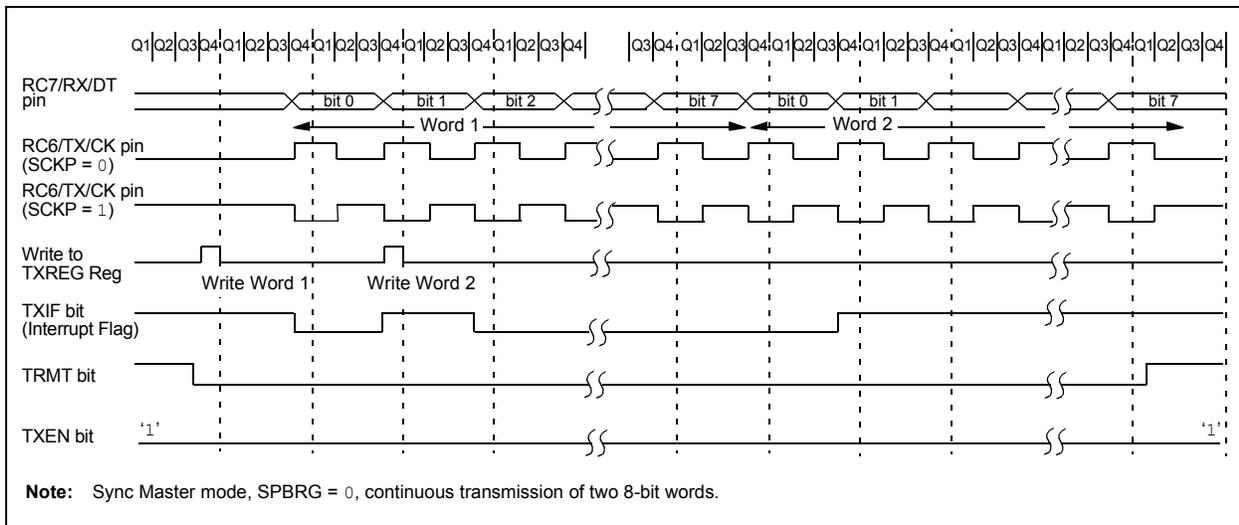
**FIGURE 17-12: SYNCHRONOUS TRANSMISSION (THROUGH TXEN)**
