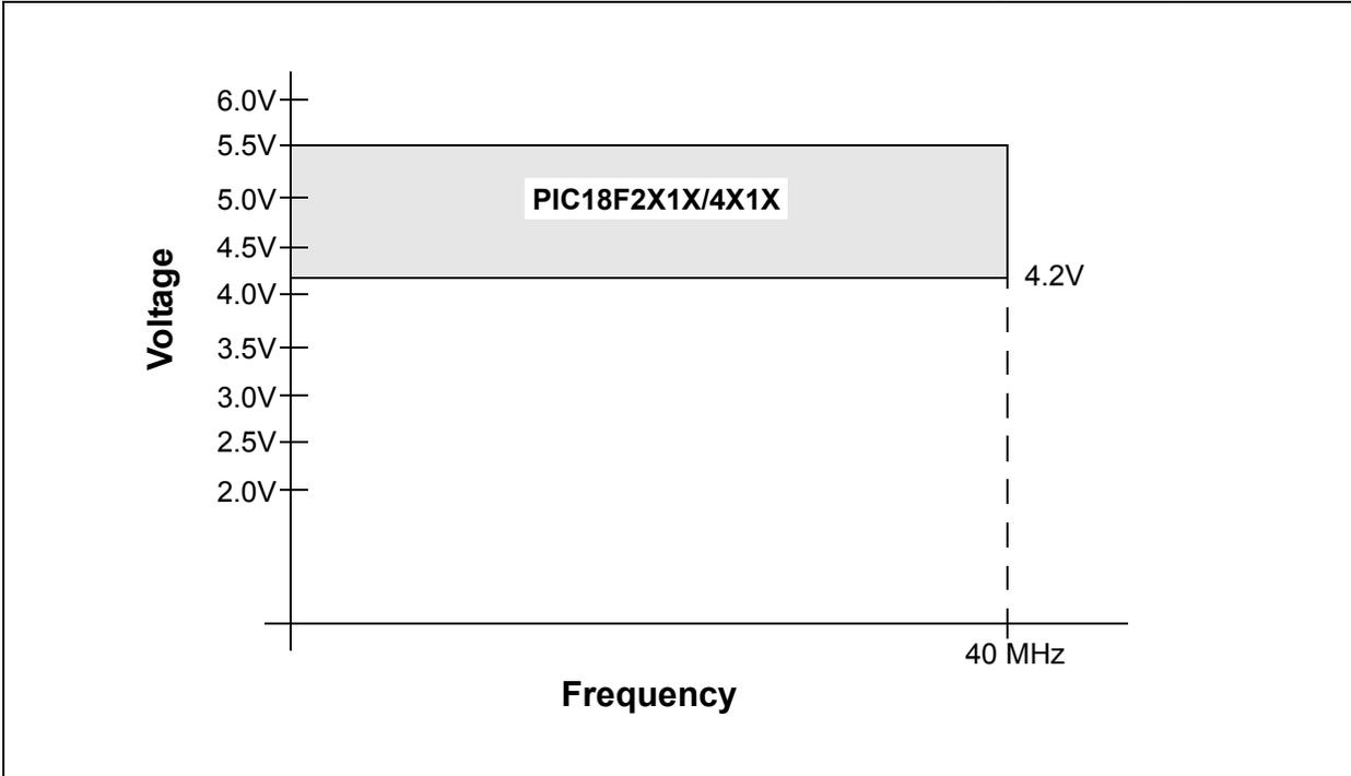
FIGURE 25-2: PIC18F2X1X/4X1X VOLTAGE-FREQUENCY GRAPH (EXTENDED)
