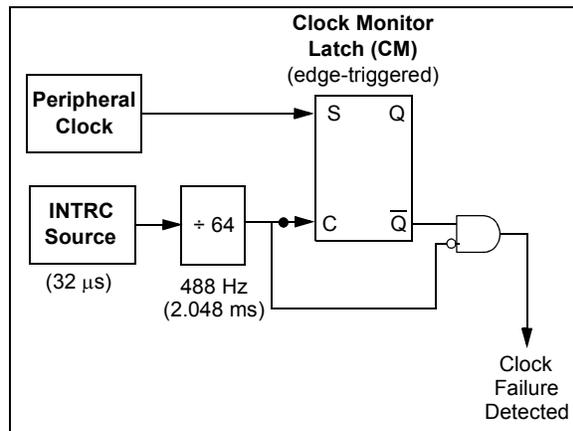
Clock failure is tested for on the falling edge of the sample clock. If a sample clock falling edge occurs while CM is still set, a clock failure has been detected (Figure 22-4). This causes the following:
