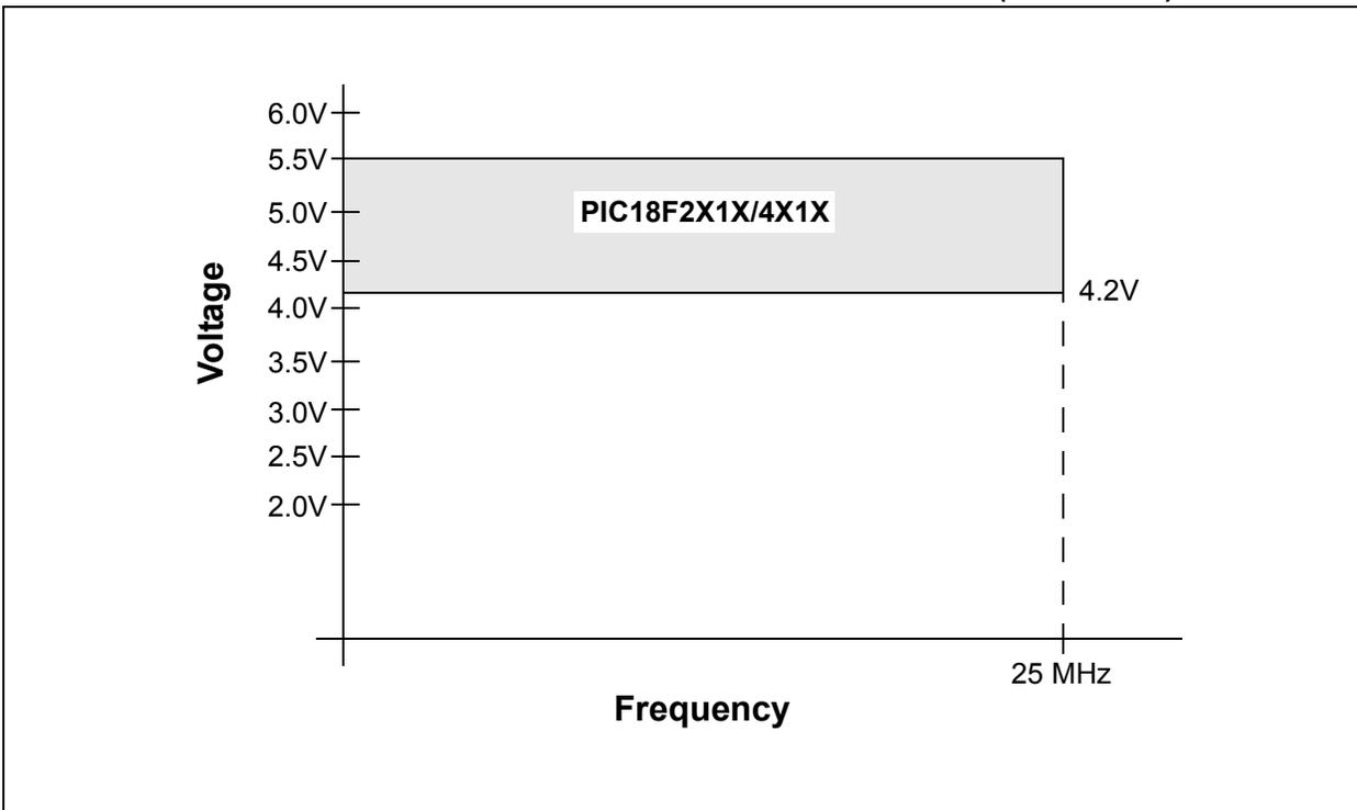
FIGURE 25-3: PIC18LF2X1X/4X1X VOLTAGE-FREQUENCY GRAPH (INDUSTRIAL)
