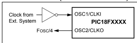
The ECIO Oscillator mode functions like the EC mode, except that the OSC2 pin becomes an additional general purpose I/O pin. The I/O pin becomes bit 6 of PORTA (RA6). Figure 2-4 shows the pin connections for the ECIO Oscillator mode.
