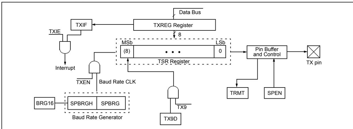
**FIGURE 17-4: ASYNCHRONOUS TRANSMISSION**
