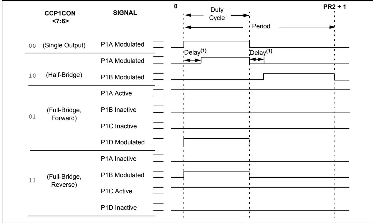
**FIGURE 15-3: PWM OUTPUT RELATIONSHIPS (ACTIVE-LOW STATE)**
