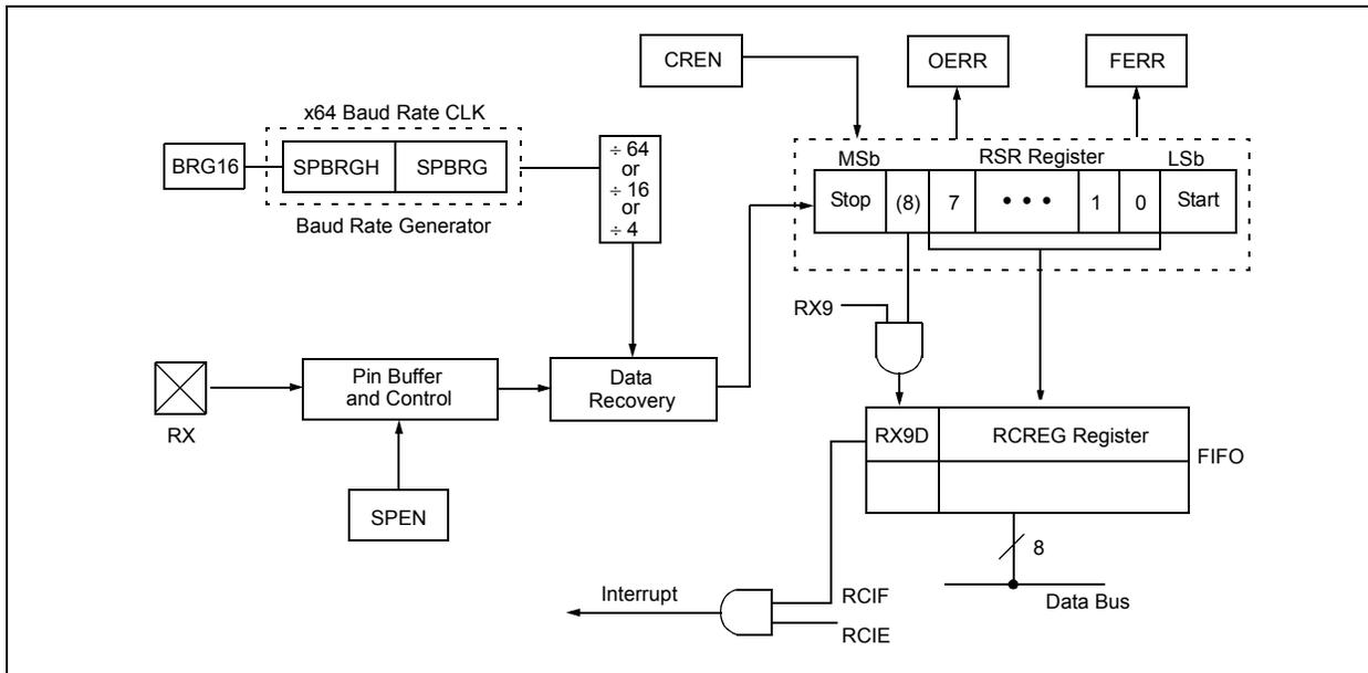
**FIGURE 17-7: ASYNCHRONOUS RECEPTION**
