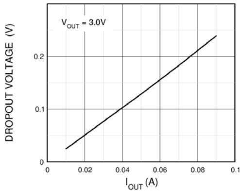
Note: Dropout voltage is defined as  $V_{CC} - V_{OUT}$  when  $V_{OUT}$  drops 3% below its nominal value.
