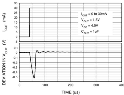
**Figure 2.10 Load Step Response— $I_{OUT} = 30mA$  to 0**
