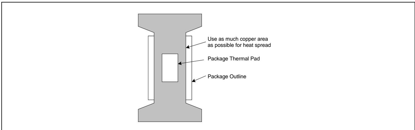
**Important:** If the attachment method is NOT implemented correctly, the functionality of the product is not guaranteed. Power dissipation capability will be adversely affected if the device is incorrectly mounted onto the circuit board.
