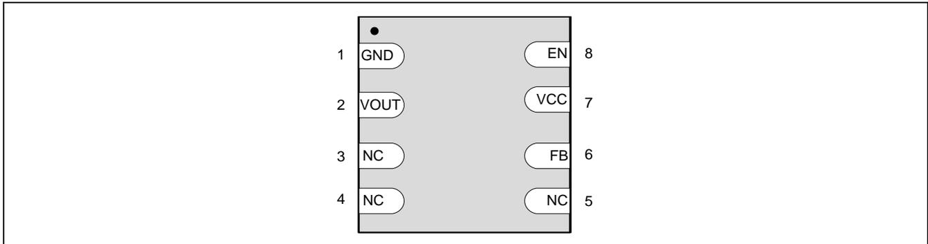
**Table 5.1 Pin Description, 8-Pin DFN (2mmx2mm)**
