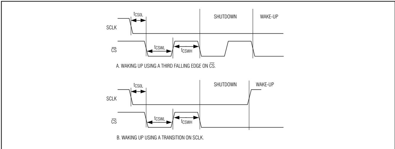
Figure 4. Shutdown Timing
