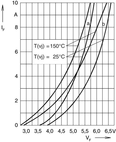
**Fig. 1: Forward characteristics**
