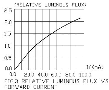
FIG.3 RELATIVE LUMINOUS FLUX VS. FORWARD CURRENT
