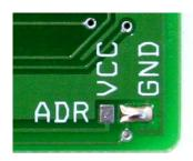
However, if you wish to connect more than two modules on the bus, the external address can be use to connect up to four modules. That is total of 16-digit. To use external address selection, remove all of the solder bridge from ADR pads. Connect voltage to the ADR pin 5 according to the table below.
