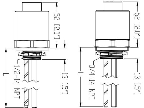
1 3/8" Power Mini 3- and 4-Pole, 10AWG, Female Receptacle, 1/2" / 3/4" NPT
