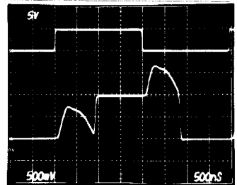
MUX-24 SMALL-SIGNAL SWITCHING WITH 2µs SAMPLE TIME
