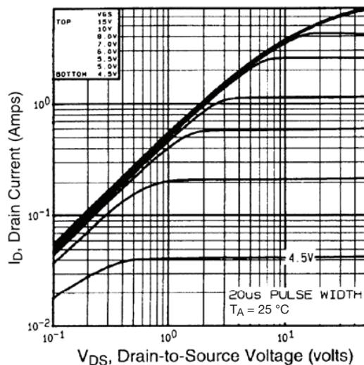
**Fig. 1 - Typical Output Characteristics,  $T_A = 25\text{ }^\circ\text{C}$**
