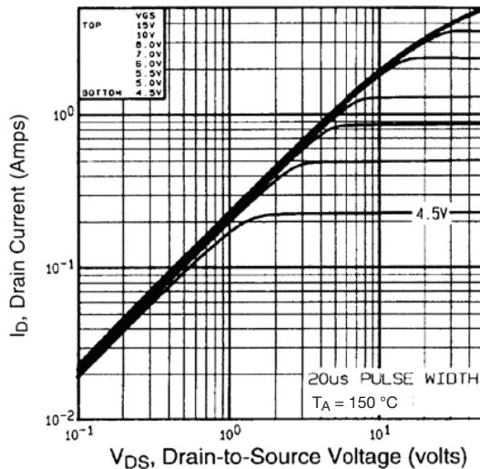
**Fig. 2 - Typical Output Characteristics,  $T_A = 150\text{ }^\circ\text{C}$**
