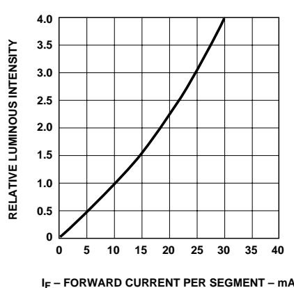
Figure 12. Relative Luminous Intensity vs. DC Forward Current.
