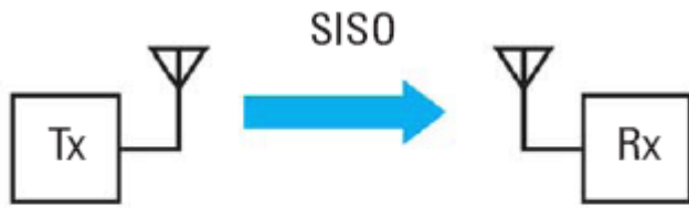
Figure 1. Single Input Single Output (SISO) radio channel access mode
