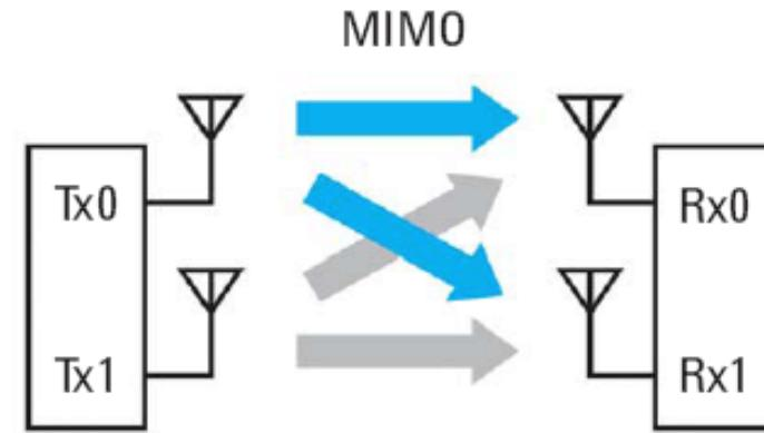
Figure 4. MIMO with two transmitters
