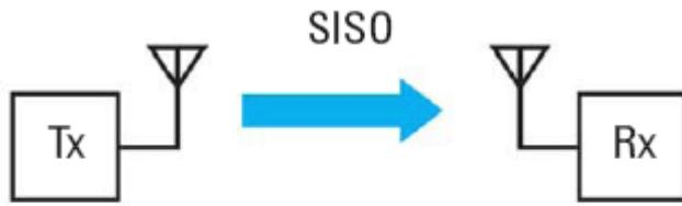
Figure 1. Single Input Single Output (SISO)
