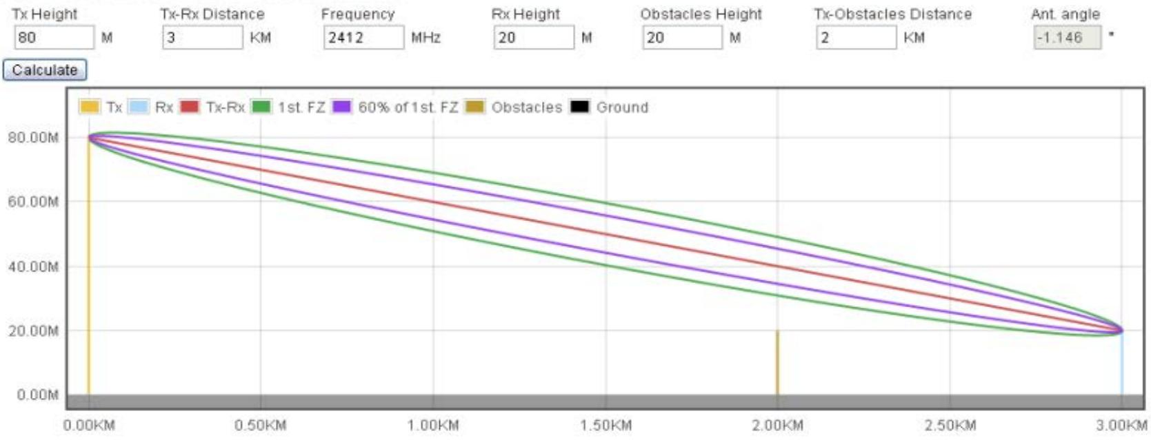
1. The Calculator can estimate the likely obstruction from existing object between two devices
