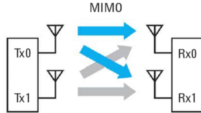
Figure 4. MIMO with two transmitters
