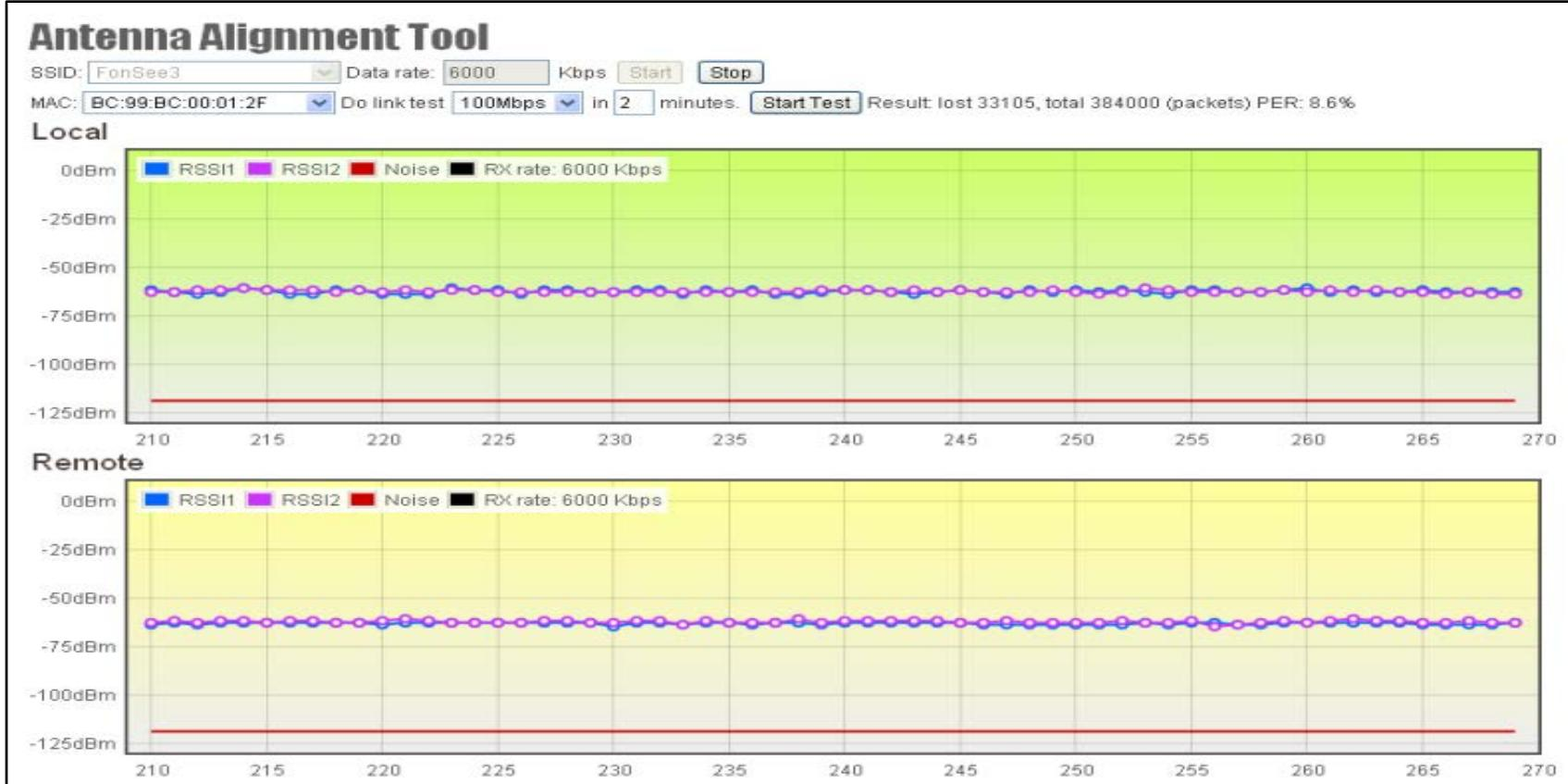
1. The tool aligns and checks the antenna directions.
