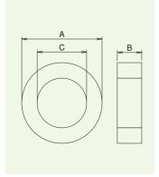
Figure 63. Toroidal type
