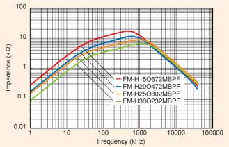
Figure 42. Frequency dependence of impedance
