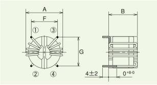
Figure 22. Single-phase VL coils
