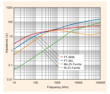
Figure 57. Frequency dependence of impedance
