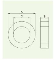
Figure 72. Toroidal type
