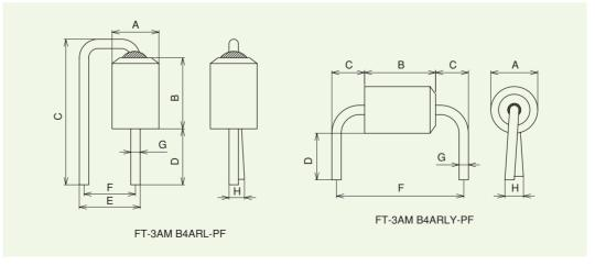
Figure 83. Lead wire core
