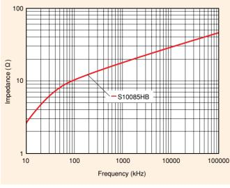
Figure 80. Frequency dependence of impedance for S10085HB
