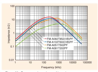
Figure 29. Frequency dependence of impedance for three-phase FM-A coils with rated current 5A-10A
