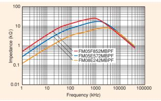
Figure 17. Frequency dependence of impedance for single-phase FM coils with rated current 5A-8A
