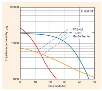
Figure 55. DC superposed characteristics of impedance permeability,  $\mu \, {\rm rz}$
