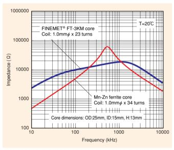
Figure 1. Comparison of impedance (8mH at 100kHz)
