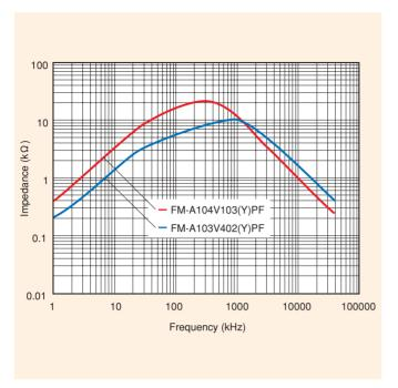
Figure 9. Frequency dependence of impedance for single-phase FM-A coils with rated current 10A
