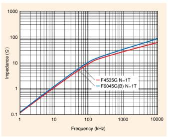
Figure 76. Frequency dependence of impedance for FT-3KL F4535G andF6045G(B)
