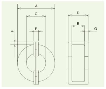
Figure 59. FT-3KL V series core
