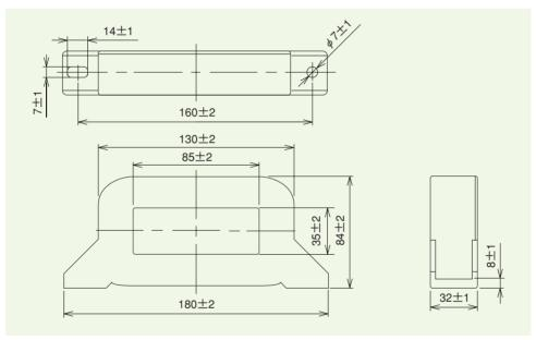
Figure 79. FT-3KL V series core
