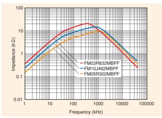
Figure 36. Frequency dependence of impedance for three-phase FM coils with rated current 3A-10A
