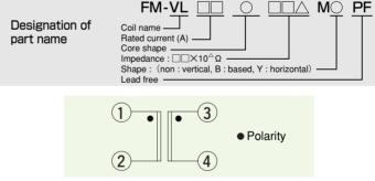
Figure 23. Circuit diagram
