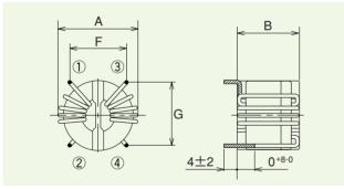
Figure 22. Single-phase VL coils
