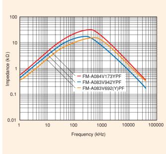
Figure 8. Frequency dependence of impedance for single-phase FM-A coils with rated current 8A
