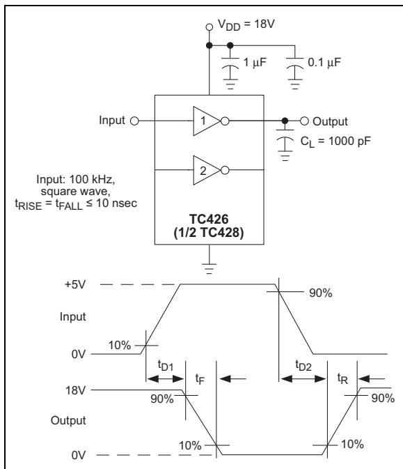
**FIGURE 3-1:** Inverting Driver Switching Time Test Circuit
