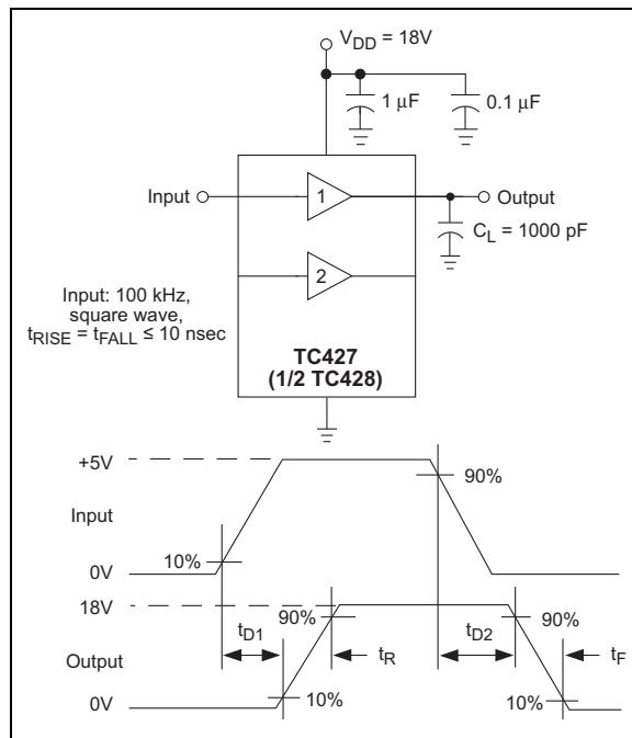
**FIGURE 3-2:** Noninverting Driver Switching Time Test Circuit
