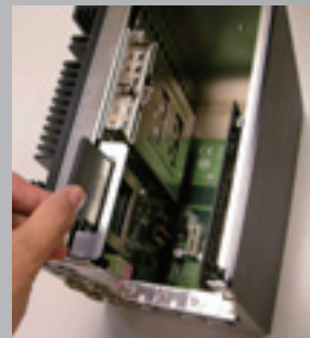
CFast Card Installation
