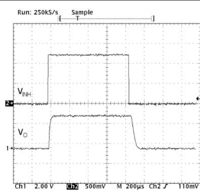
$V_I = 5\text{ V}$ ,  $I_O = 1\text{ mA}$ ,  $V_{INH} = 0$  to  $1.2\text{ V}$ ,  $C_I = C_O = 1\text{ }\mu\text{F}$  (cer),  $C_{BYP} = 10\text{ nF}$ ,  $T_R = T_F = 1\text{ }\mu\text{s}$
