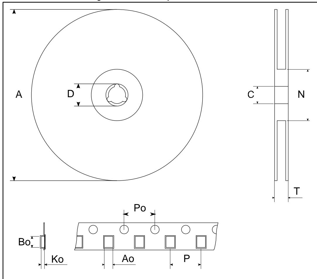
Table 8: SOT23-5L tape and reel mechanical data
