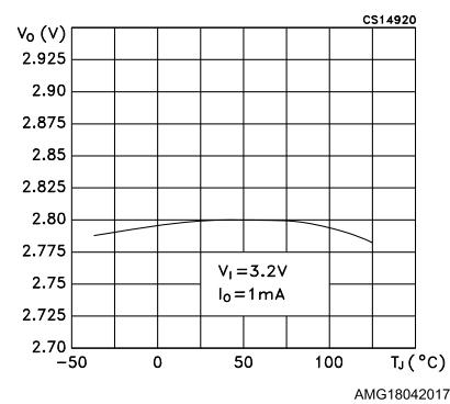
**Figure 5: Output voltage vs temperature  $V_O = 3.3\text{ V}$**
