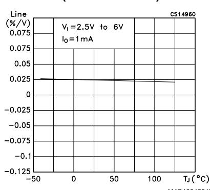
**Figure 9: Line regulation vs temperature
