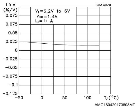
**Figure 10: Line regulation vs temperature
