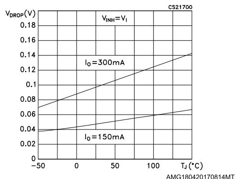
**Figure 16: Dropout voltage vs output current**
