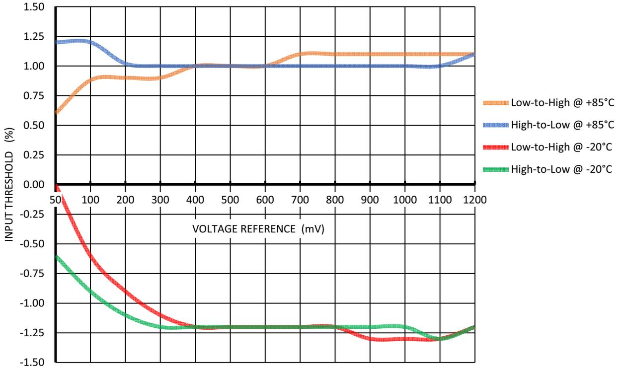
Figure 20. Input Threshold Ratio vs. Voltage Reference at VDD = (1.71 - 5.5) V, V<sub>hys</sub> = 0, Gain = 1
