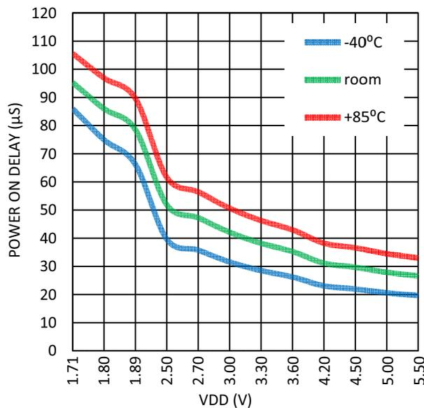
**Figure 15. Maximum Power On Delay vs. VDD.**
