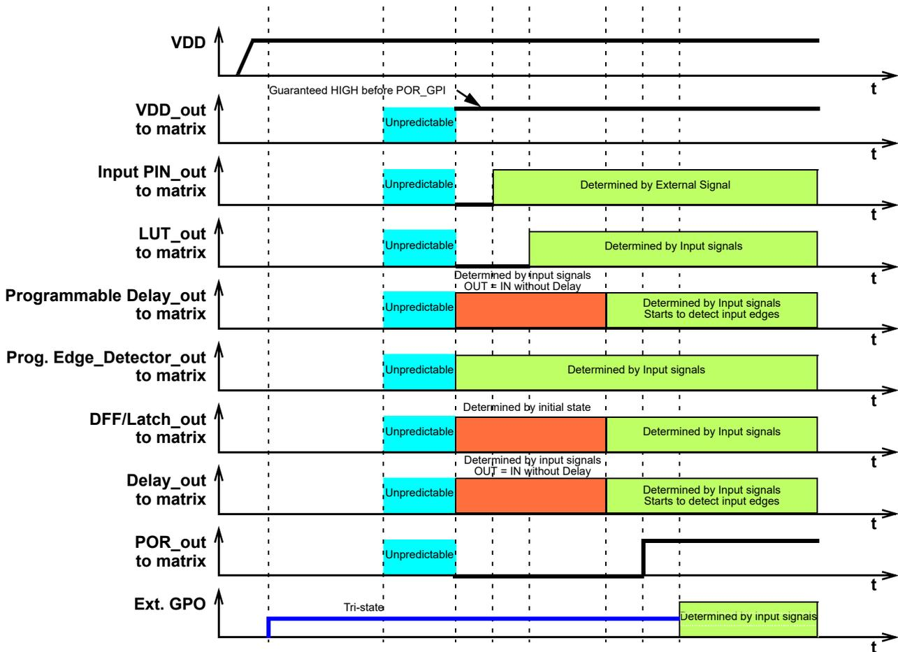
Figure 44. Internal Macrocell States during POR sequence
