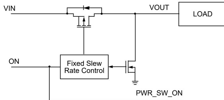
Figure 45. P-FET Power Switch with Slew Rate Control
