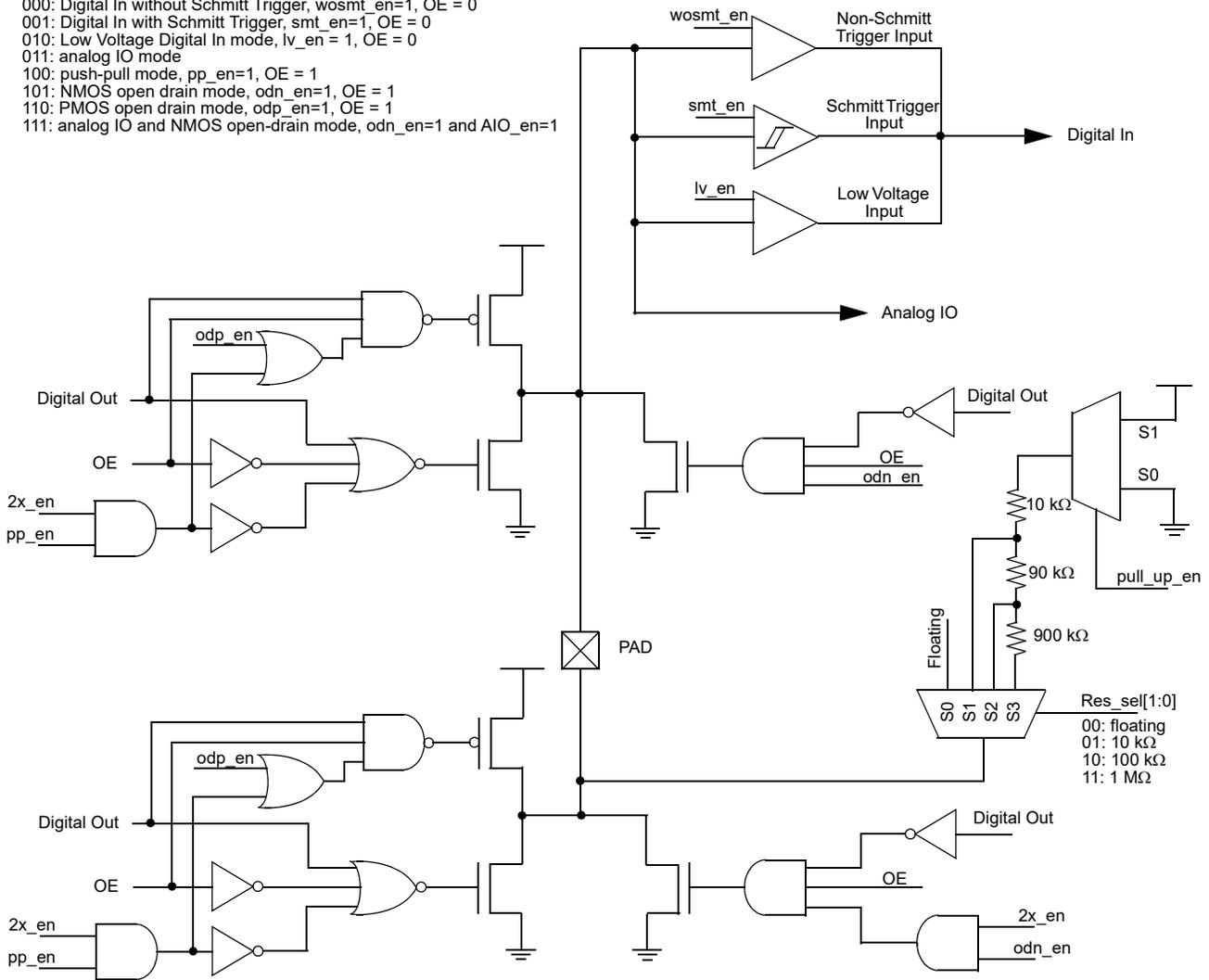
Figure 4. Register OE IO Structure Diagram
