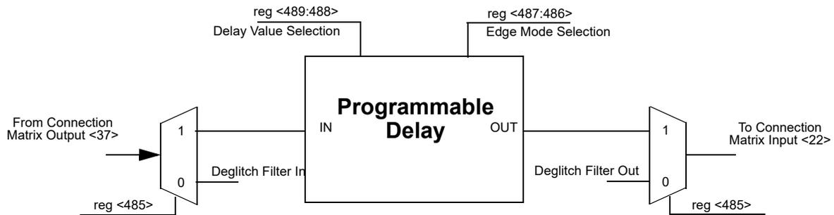
Figure 35. Programmable Delay
