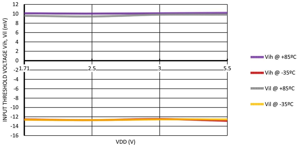
Figure 21. Input Threshold Voltage V<sub>ih</sub>, V<sub>il</sub> vs. VDD at V<sub>ref</sub> = 1000 mV, Gain = 1
