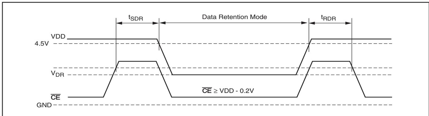
**DATA RETENTION SWITCHING CHARACTERISTICS (LOW POWER) (IS61/64C5128AS)**
