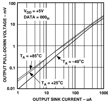
Figure 6. Pull-Down Voltage vs. Output Sink Current Capability
