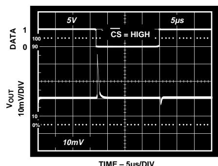
Figure 22. Digital Feedthrough vs. Time
