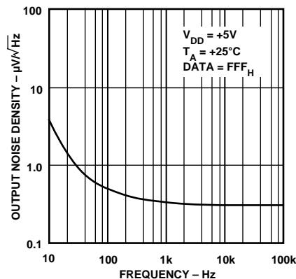
Figure 18. Output Voltage Noise Density vs. Frequency
