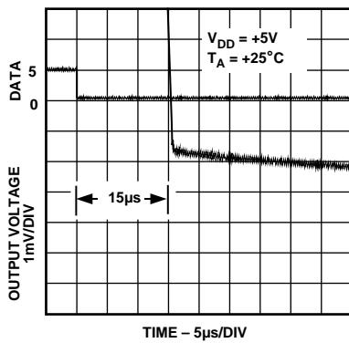
Figure 14. Output Voltage Fall Time Detail
