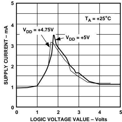
Figure 9. Supply Current vs. Logic Input Voltage
