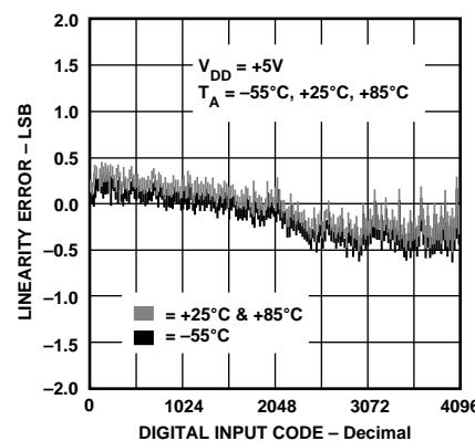
*Figure 2. Linearity Error vs. Digital Code and Temperature*
