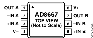
Figure 3. 8-Lead MSOP (RM-8), 8-Lead SOIC (R-8)
