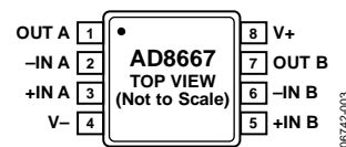
Figure 3. 8-Lead MSOP (RM-8), 8-Lead SOIC (R-8)
