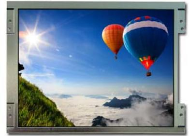
Kyocera offers three versions of 8.4" VGA TFT LCDs: the AN00 is the normal brightness version with 450nits brightness; the AN20 has the CCC ( constant current circuit) built-in, and the AN50 is the high brightness version with 850nits brightness, ideal for outdoor applications. All three products features long life LED with 70K hours lifetime, wide operating temperature range, standard CMOS interface.
