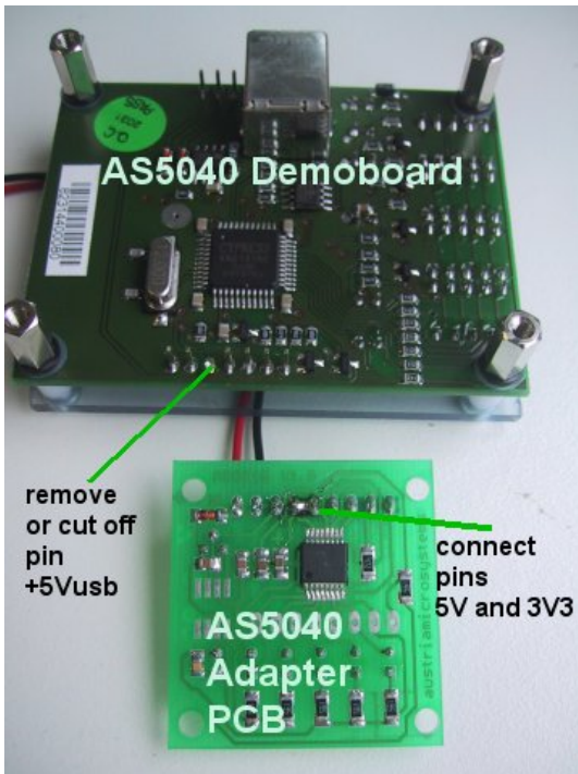
Figure 9: configuring the Adapter PCB for 3.3V operation
