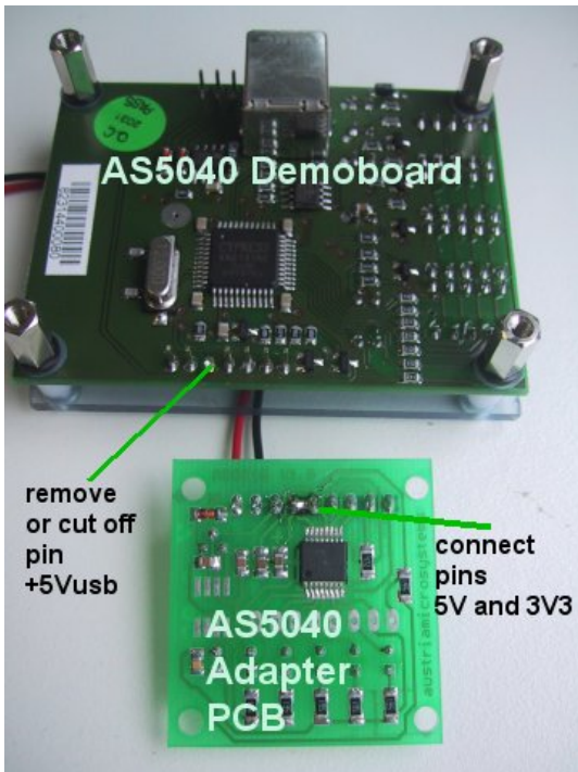
Figure 9: configuring the Adapter PCB for 3.3V operation
