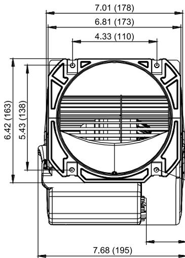
4x sheet metal nut for EN ISO 1478-ST4,8 thread. Screw length 0.5 in (12.5 mm)
