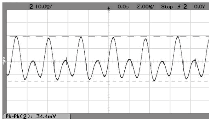
Output Ripple and Noise (Vin=5V, Vout=1.8V, Iout=3A, Cloud=0, ScopeBW=100MHz)
