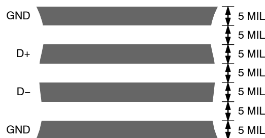
Figure 23. Typical Arrangement of Signal Tracks
