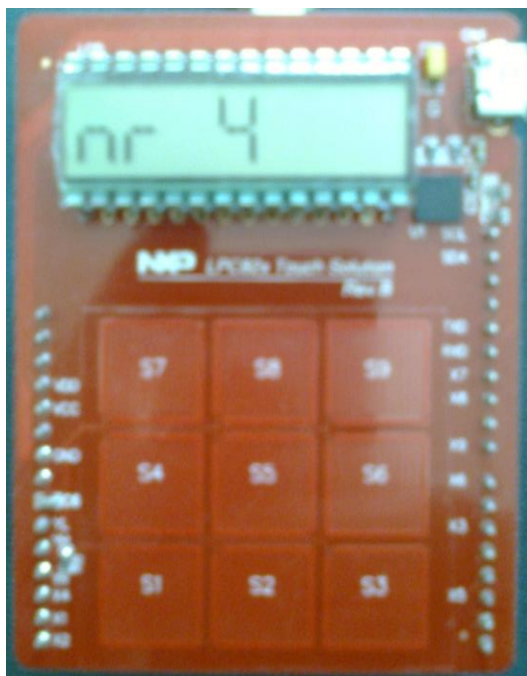
Fig 6. Gesture recognition by LPC824 target
