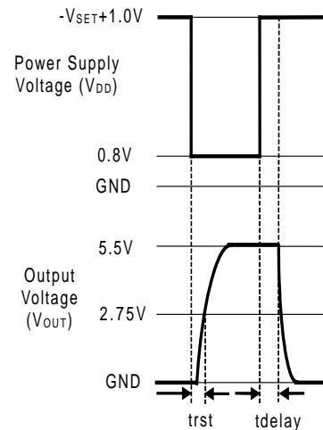
**Figure 10. Nch Open Drain Inverting Output**
