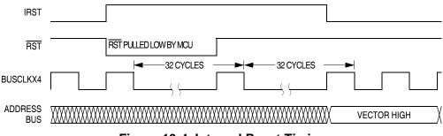
Figure 13-4. Internal Reset Timing
