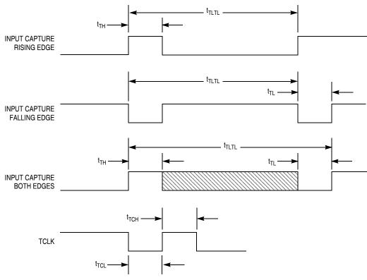
Figure 16-11. Timer Input Timing
