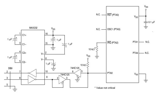
Figure 15-12. Monitor Mode Circuit (Internal Clock, No High Voltage)
