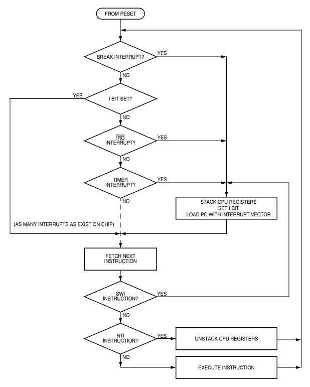
Figure 13-7. Interrupt Processing
