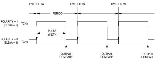
Figure 14-3. PWM Period and Pulse Width
