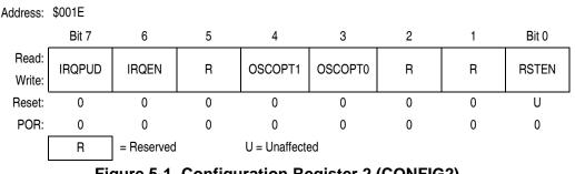
Figure 5-1. Configuration Register 2 (CONFIG2)
