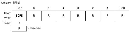
Figure 15-8. Break Flag Control Register (BFCR)
