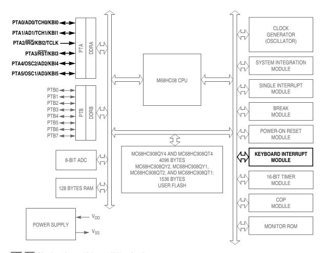
RST, IRQ: Pins have internal (about 30K Ohms) pull upPTA[0:5]: High current sink and source capabilityPTA[0:5]: Pins have programmable keyboard interrupt and pull upPTB[0:7]: Not available on 8-pin devices – MC68HC908QT1, MC68HC908QT2, and MC68HC908QT4 (see note in12.1 Introduction)
