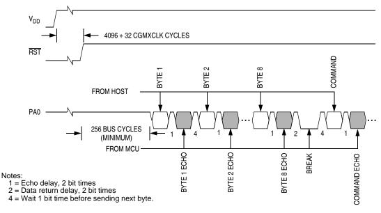
Figure 15-18. Monitor Mode Entry Timing
