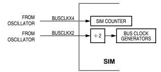
Figure 13-2. SIM Clock Signals
