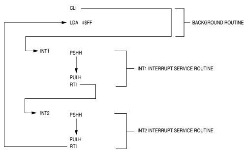
Figure 13-10. Interrupt Recognition Example
