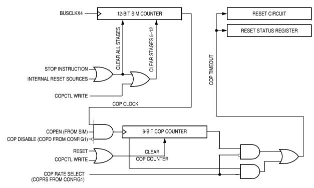
Figure 6-1. COP Block Diagram
