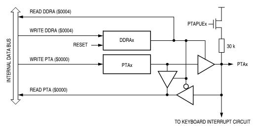
Figure 12-3. Port A I/O Circuit
