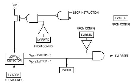
Figure 10-1. LVI Module Block Diagram
