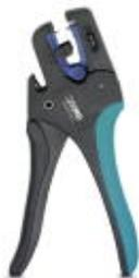
Stripping tool, for cables and conductors (especially for rubber and silicone insulations) from 0.1 - 4 mm<sup>2</sup>, self-adjusting, stripping length of up to 18 mm, cutting capacity of up to 10 mm<sup>2</sup> stranded/1.5 mm<sup>2</sup> solid, replaceable stripping blade
