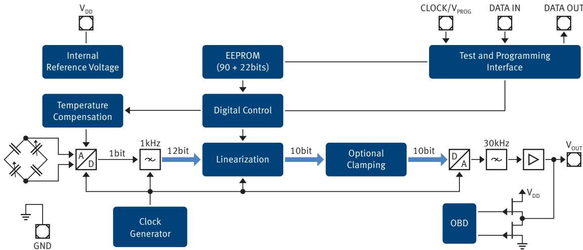
Infineon offers an extensive broad product portfolio for diesel engine management systems from micro-machined sensors to smart power ICs and microcontrollers. The KP21x pressure sensor as an integrated pressure sensor for manifold pressure measurement is a benchmark in terms of reliability, performance and integration level.
