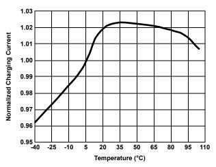
Figure 6. Charge Current vs Temperature
