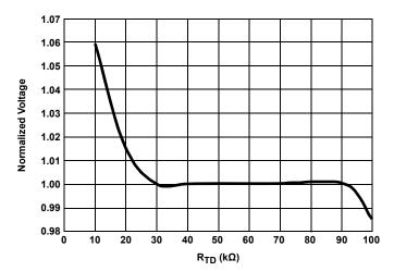
Figure 7. Timing Capacitor Voltage vs R<sub>TD</sub>
