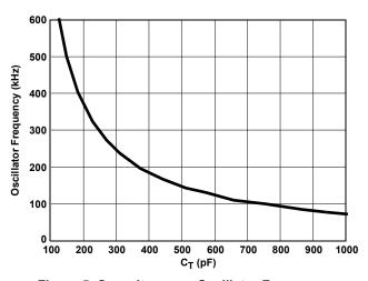
Figure 5. Capacitance vs Oscillator Frequency  $(R_{TD} = 49.9k\Omega)$
