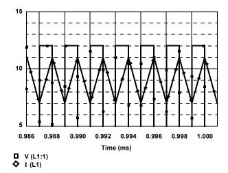
Figure 16. Steady State Secondary Winding Voltage and Inductor Current
