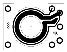
Figure 9. Top Layer: 1 Turn Secondary and SR Windings
