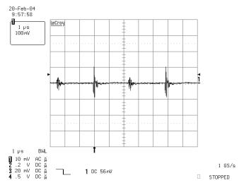
Figure 21. Output Ripple and Noise - 20MHz BW
