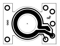
Figure 14. Bottom Layer: 1 Turn Secondary and SR **Windings**
