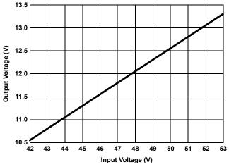
Figure 20. Line Regulation at I<sub>OUT</sub> = 1A
