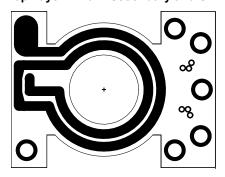
Figure 11. Internal Layer 2: 2 Turns Primary Winding
