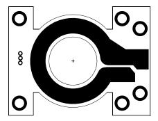
Figure 13. Internal Layer 4: 1 Turn Secondary Winding
