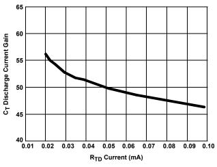
Figure 3. Oscillator C<sub>T</sub> Discharge Current Gain
