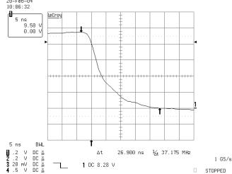
Figure 23. FET Drain-Source Voltage Near-ZVS Transition
