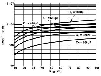
Figure 4. Dead Time vs Capacitance
