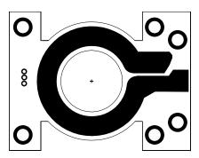
Figure 10. Internal layer 1: 1 Turn Secondary Winding
