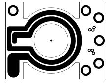
Figure 12. Internal Layer 3: 2 Turns Primary Winding
