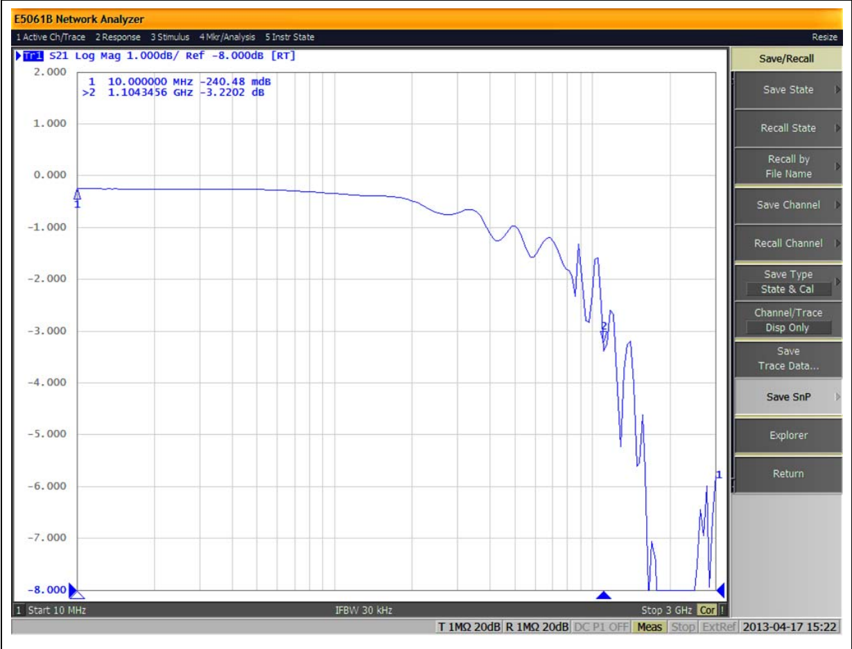
Figure 17. Data switch transfer characteristics vs. frequency
