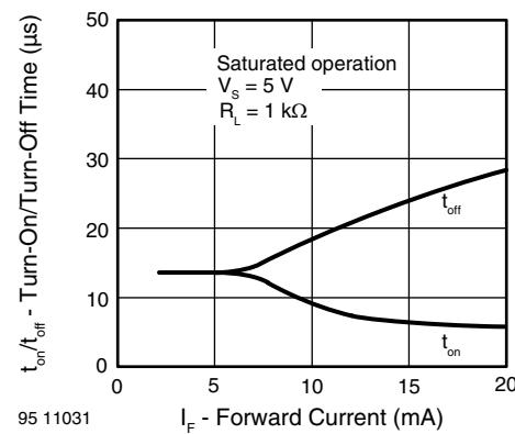
Fig. 18 - Turn-On/Turn-Off Time vs. Forward Current
