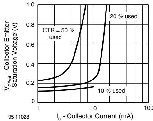
Fig. 17 - Collector Emitter Saturation Voltage vs. Collector Current
