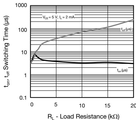
Fig. 16 - Switching Time vs. Load Resistance
