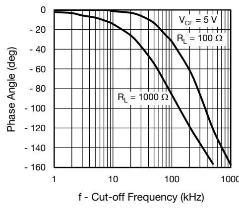
Fig. 14 -  $f_{CTR}$  vs. Phase Angle
