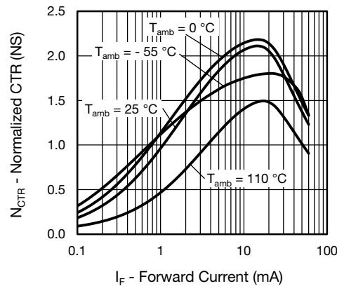
Fig. 12 - Current Transfer Ratio vs. Forward Current (saturated)
