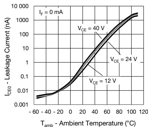
Fig. 8 - Collector Emitter Current vs. Ambient Temperature
