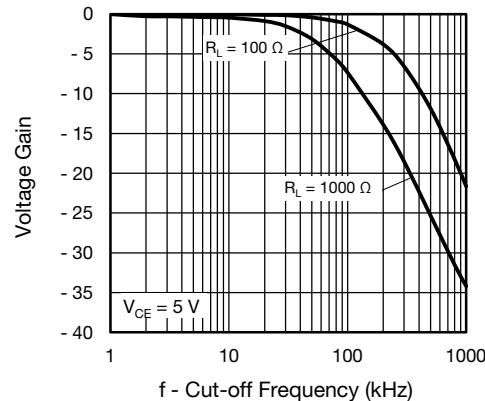
Fig. 19 - Voltage Gain vs. Cut-off Frequency
