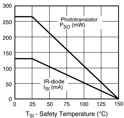
Fig. 4 - Derating Diagram
