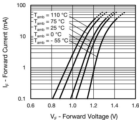
Fig. 6 - Forward Voltage vs. Forward Current
