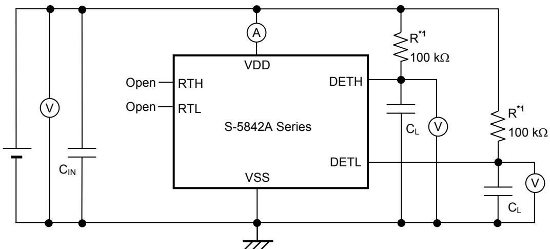
\*1. Resistor (R) is unnecessary for the CMOS output product.
