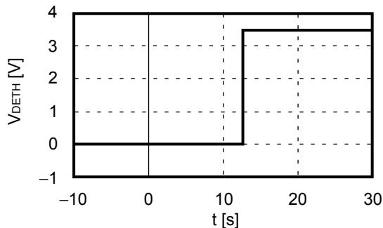
**5. 2 When SNT-6A is put into the liquid of +100°C from the air of +25°C at t = 0 s**
