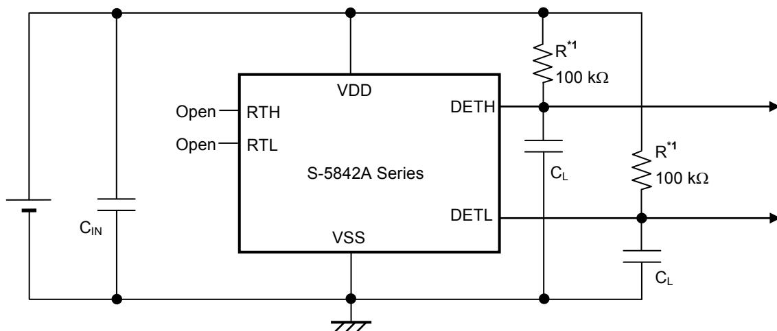
\*1. Resistor (R) is unnecessary for CMOS output product.
