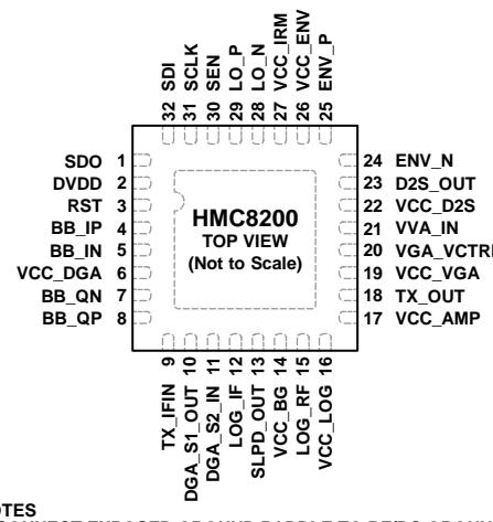
Figure 2. Pin Configuration
