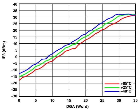
Figure 40. Output IP3 vs. DGA Word over Temperature, RF = 1 GHz, Measurement Conducted with VCC\_VGA = 3.3 V (Maximum Gain) on RF VGA
