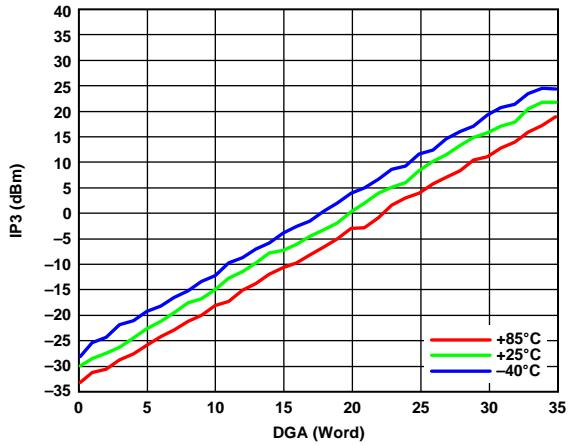
Figure 41. Output IP3 vs. DGA Word over Temperature, RF = 4 GHz, Measurement Conducted with VCC\_VGA = 3.3 V (Maximum Gain) on RF VGA
