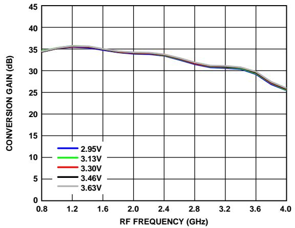
Figure 20. Conversion Gain vs. RF Frequency at Various V<sub>CCX</sub>
