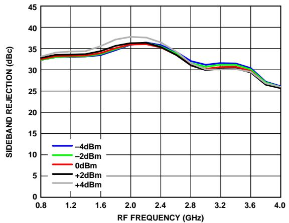
Figure 18. Sideband Rejection vs. RF Frequency at Various LO Powers
