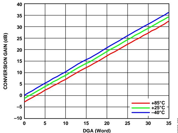
Figure 33. Conversion Gain vs. DGA Word over Temperature, RF = 1 GHz,
