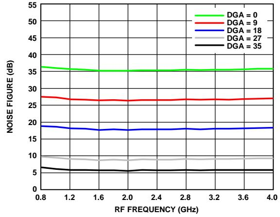
Figure 44. Noise Figure vs. RF Frequency over DGA Word at VCC\_VGA = 3.3 V
