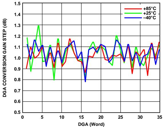
Figure 39. Conversion Gain Step vs. DGA Word over Temperature, RF = 4 GHz
