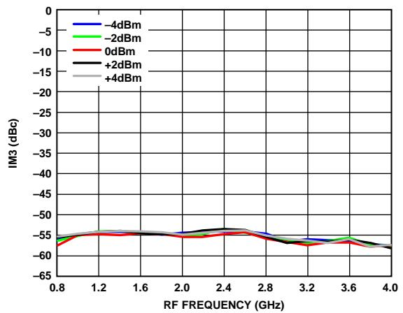
Figure 19. IM3 vs. RF Frequency at Various LO Powers
