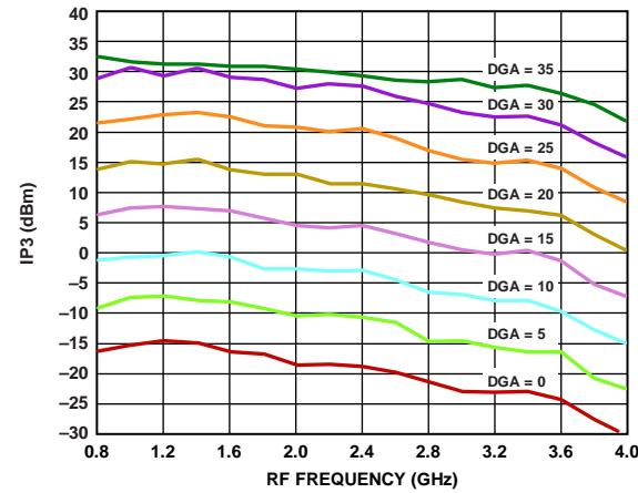
Figure 37. Output IP3 vs. RF Frequency over DGA Word, Measurement
