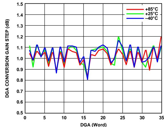
Figure 36. Conversion Gain Step vs. DGA Word over Temperature,
