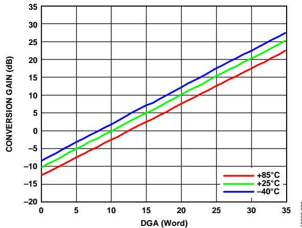
Figure 34. Conversion Gain vs. DGA Word over Temperature, RF = 4 GHz,
