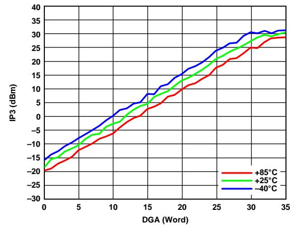
Figure 38. Output IP3 vs. DGA Word over Temperature, RF = 2 GHz,
