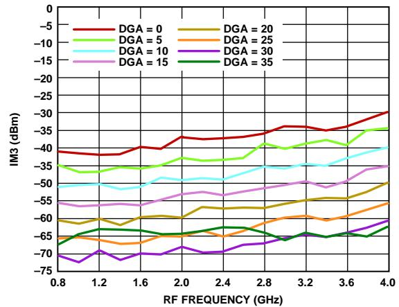
Figure 42. IM3 vs. RF Frequency over DGA Word, Measurement Conducted with VCC\_VGA = 3.3 V (Maximum Gain) on RF VGA
