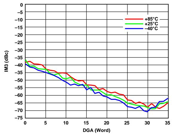
Figure 43. IM3 vs. DGA Word over Temperature, RF = 2 GHz, Measurement Conducted with VCC\_VGA = 3.3 V (Maximum Gain) on RF VGA
