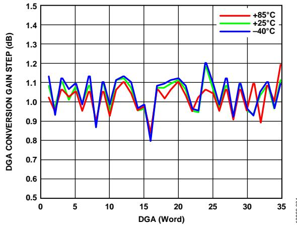
Figure 35. Conversion Gain Step vs. DGA Word over Temperature, RF =
