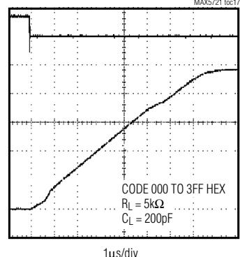
**FULL-SCALE SETTLING TIME ( $V_{DD} = +5\text{V}$ )**
