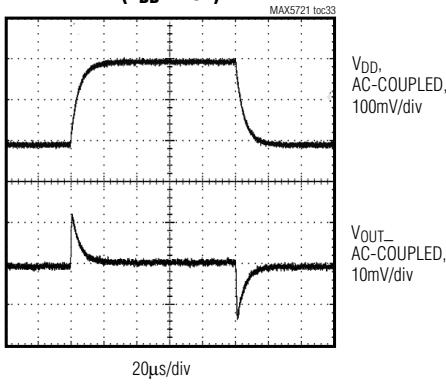
**LINE TRANSIENT RESPONSE ( $V_{DD} = +5\text{V}$ )**
