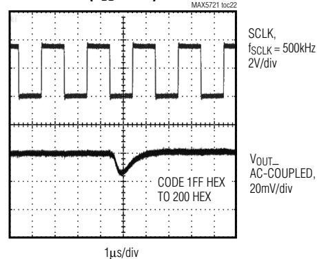
**DIGITAL-TO-ANALOG GLITCH IMPULSE ( $V_{DD} = +3\text{V}$ )**
