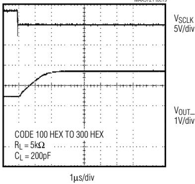
**HALF-SCALE SETTLING TIME ( $V_{DD} = +3\text{V}$ )**
