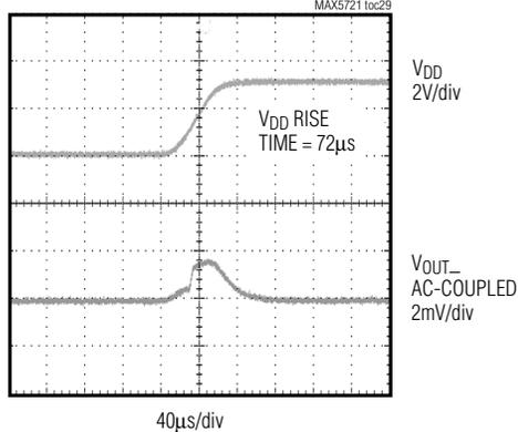
**CLOCK FEEDTHROUGH ( $V_{DD} = +5\text{V}$ )**
