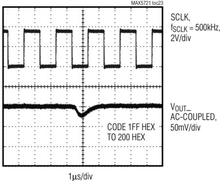
**DIGITAL-TO-ANALOG GLITCH IMPULSE ( $V_{DD} = +5\text{V}$ )**
