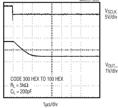
**EXITING POWER-DOWN ( $V_{DD} = +5\text{V}$ )**
