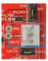
By default, the jumpers J16 and J7 are populated. These connect pin 3 (VBAT1) of the LIN1 connector and pin 3 (VBAT2) of the LIN2 connector to the VIN power rail of the Shield Kit, respectively. This is useful if you want to power up other LIN nodes/analyzers through either of the LIN connectors, or if you want to power the Pioneer Kit and shield board from the power supply (12 V) of some other LIN node (LIN analyzer).
