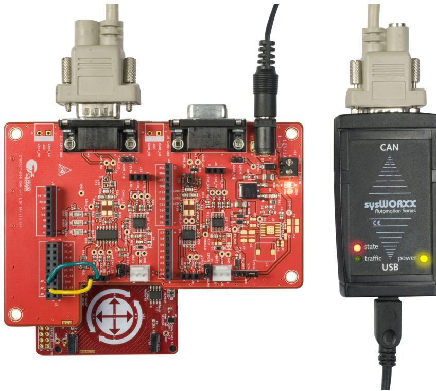
Figure 4-2. CAN Analyzer Connection to CY8CKIT-026's CAN1 Transceiver
