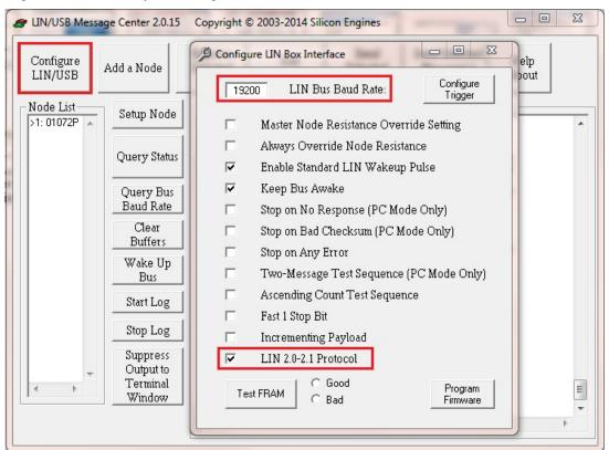
5. If you are using any other analyzer, make sure that the checksum setting is selected as enhanced checksum since LIN v2.1/2.2 specification supports only enhanced checksum (this option is not required in Silicon Engines LIN-USB converter software).
