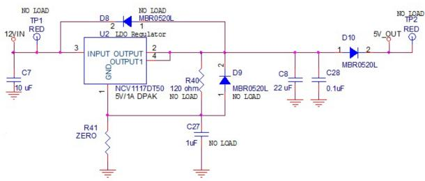
**Warning:** The regulator can support up to 1 A current, connecting this to any circuit which draws more than 1 A current will damage the regulator. Do not provide any power through the test points.
