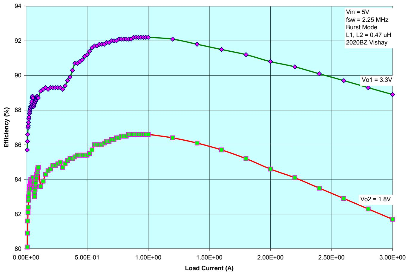
Figure 6. LTC3615 DC1572 Efficiency
