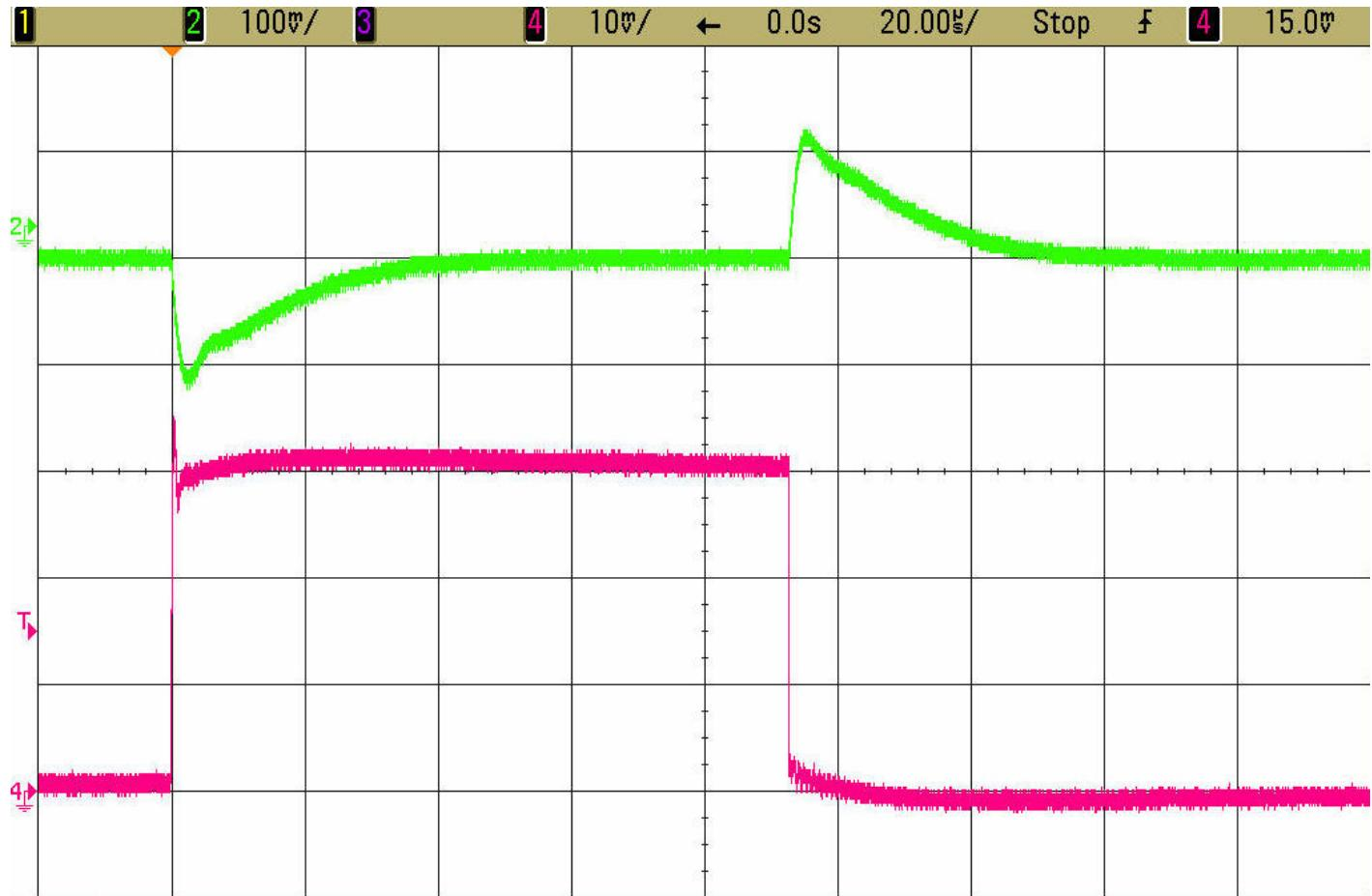
Figure 3.  $V_{OUT1}$  Load Step Response
