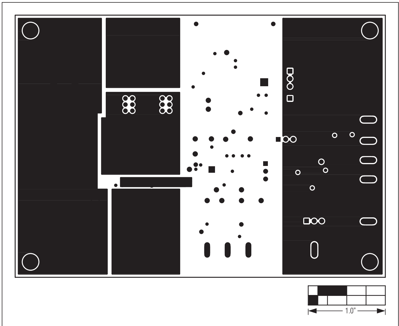
Figure 5. MAX5977A EV Kit PCB Layout—Inner Layer 3
