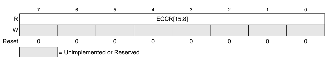
Figure 19-20. Flash ECC Error Results High Register (FECCRHI)
