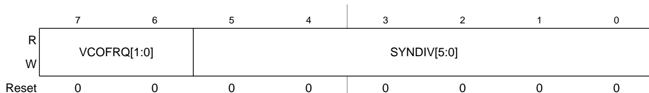
Figure 8-3. S12XECRG Synthesizer Register (SYNR)
