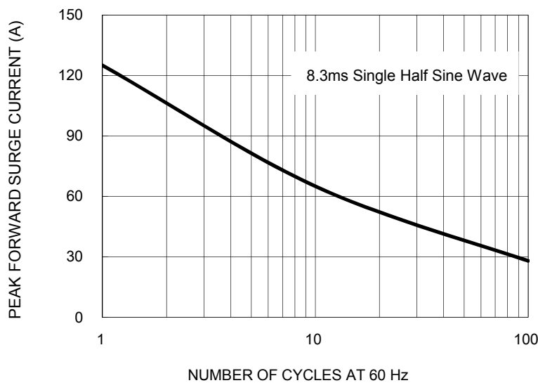
FIG. 3 MAXIMUM NON-REPETITIVE FORWARD SURGE CURRENT
